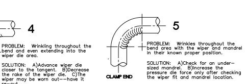
After the initial tooling set-up has been made, make a sample bend to determine what tools to adjust in order to make a better bend. It is important to keep in
