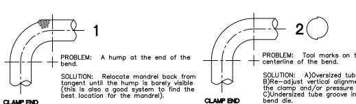
Start with a clean, débur and lubricated tube with elongation properties sufficient to produce the bend.
