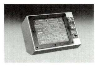
233 Control. Three bend modes are available. They are manual, semi-automatic (with or without the carriage) and syncro semi-automatic (with the carriage). The 233 controller has the capacity for 100 programs consisting of 1 to 10 bends (DOB) per program. Each control function has a light that informs the operator when the function is activated or complete.
