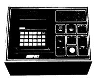
**210-HR Control.** Three bend modes are available. They are manual, semi-automatic (with or without the carriage), and synchro semi-automatic (with the carriage). The 210-HR controller has the capacity for 100 programs consisting of 1 to 10 bends (DOB's) per program.
