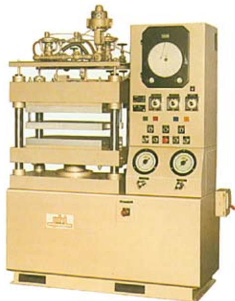
Pictured is Model No. 75R2418-3 Steam heated platens
