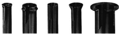
FLARING BEADING SQUARING DOUBLE FLARING FLANGING
